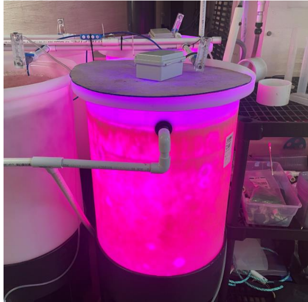
Fig. 25. Core-lit tumble culture with adjustable lights.
