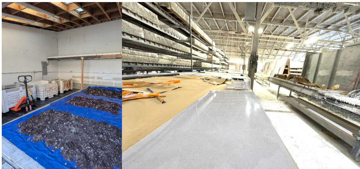
Figure 44. Primitives MARBLIS manufacturing trial successfully converted raw dried sea urchin into large proof of concept Urchinite slabs at manufacturing plant.
